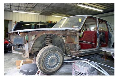
Lack of commonality with other Triumphs makes restoration of a 2000 challenging. A few Triumph 2000 Mk Is were imported to the United States, but the body was restyled for the Mk II. Doors are the same, and most underskin parts are similar, but finding 2000 parts in the United States is nearly impossible. Triumph did not ex-
